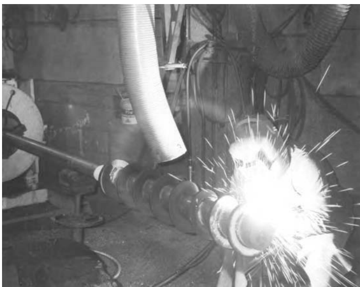
Installing Flights by Arc Welding
