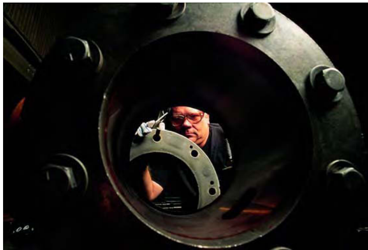
Upon receipt, compressor is disassembled and each component is thoroughly inspected.
